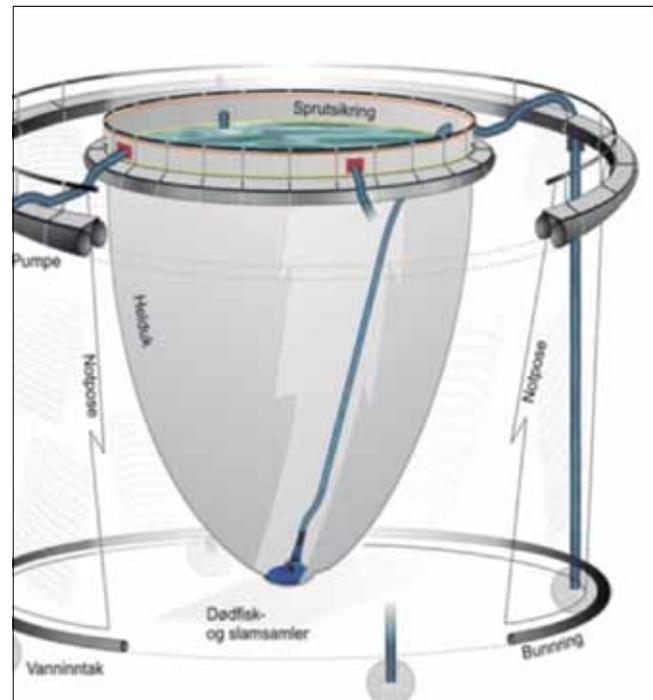
Figura 9. Closed bag (Fuente : Akva-Design)
